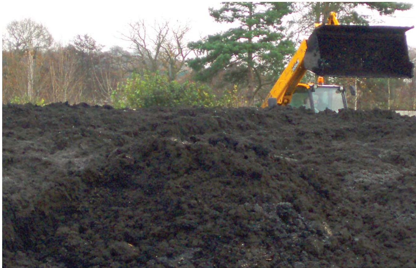
A sludge cake stockpile
